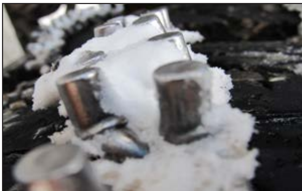
Above: Close-up of our Nordic 8mm studs after 500 kms of use on a loaded tandem-trailer logging truck .
