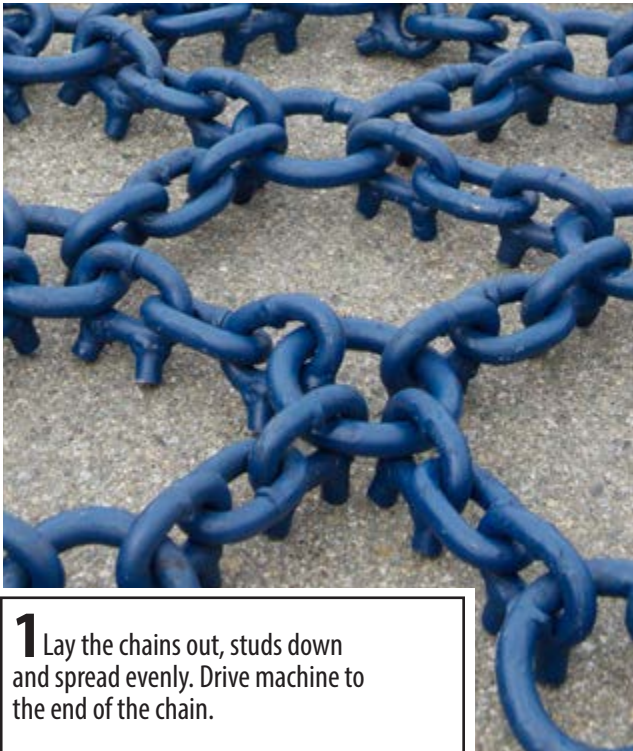
Netlink Style Chain INSTALLATION GUIDE
